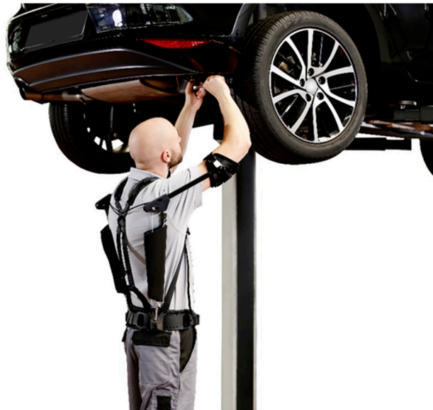
Figure 1. The passive exoskeleton Paexo used in industrial environment.
