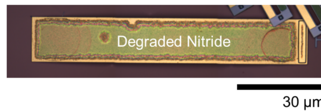
Figure 4. Optical microscope image of a polysilicon cantilever coated with Au and the post-processed silicon nitride layer after release in hydrofluoric acid (49%) Degradation of the nitride is evident.
