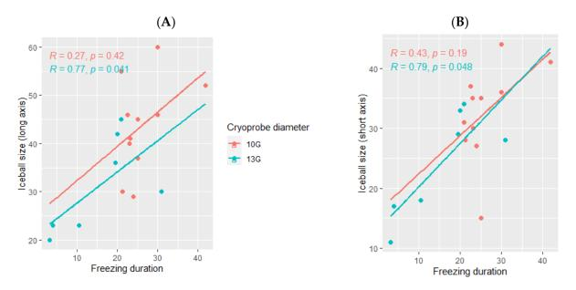
**Figure 4.** Correlation between the ice ball size and the total freezing duration, depending on the cryoprobe used (10G: orange; 13G: blue); (**A**): major axis; (**B**): minor axis. The correlations are represented by the Spearman coefficient (R). A coefficient close to 1 shows a strong positive correlation, while a coefficient close to -1 shows a strong negative correlation. The *p*-value (*p*) indicates the significance level of the observed correlation.
