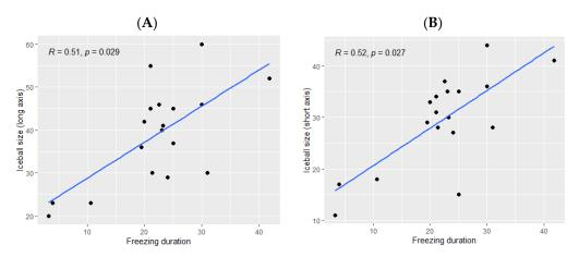
**Figure 2.** Correlation between the ice ball size and the total freezing duration; (**A**): major axis; (**B**): minor axis. The correlations are represented with Spearman coefficient (R). A coefficient close to 1 shows a strong positive correlation, while a coefficient close to -1 shows a strong negative correlation. The *p*-value (*p*) indicates the significance level of the observed correlation.
