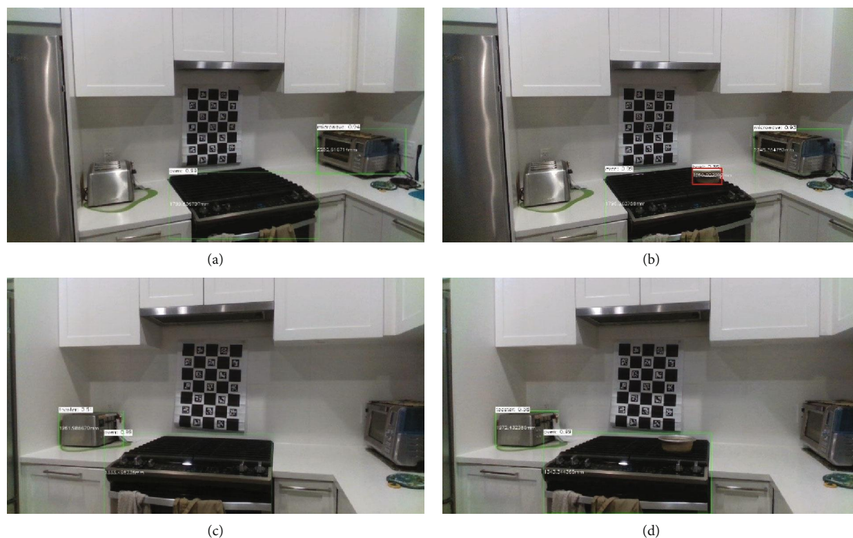
FIGURE 11: Object detection for before and after the instances when an older adult walks in the kitchen monitoring area and places a cooking bowl on the oven. Left column (a, c) is the detected objects from left (a) and right (c) sensors before an older adult walks into the scene. The right column (b, d) is the detected objects from the left (b) and right (d) sensors when the older adult leaves the scene. Notice the bowl was not detected in the view of the right sensor for when the older adult leaves the room. However, calibration results are used to segment the point cloud in view of the right sensor.
