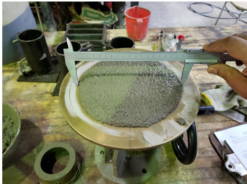
Figure 2. Evaluation of the workability performance of prepared mortars.
