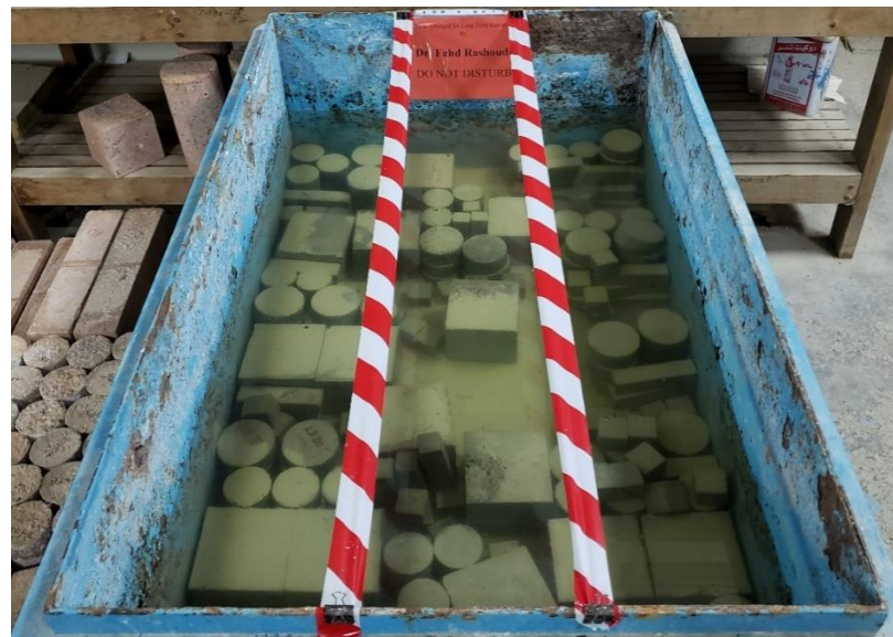
Figure 1. Curing condition of proposed mortar specimens.
