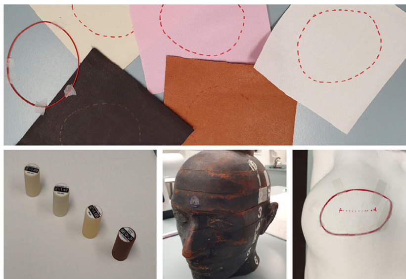
Figure 1. Top, wire and ink markings; bottom left-to-right, Gammex rods, RANDO phantom, plaster breast phantom.
