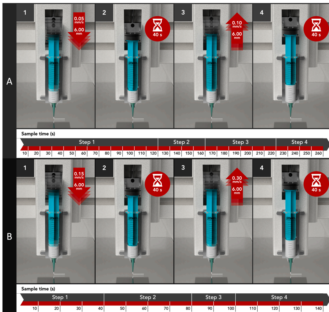
Fig. 2. Diagram of compression/shrinkage cycle, showing the two extrusion speeds tested: A) 0.05 mm/s and B) 0.15 mm/s.
