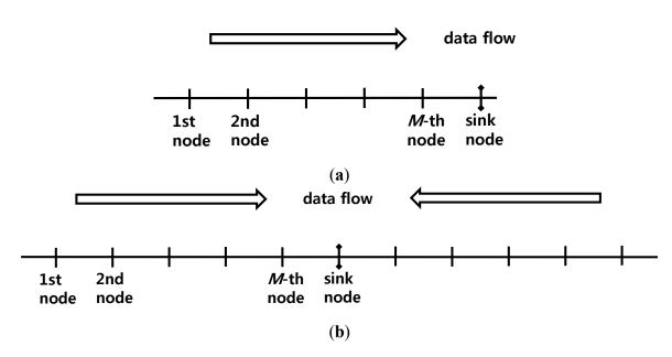
Figure 3. One-dimensional linear data flow. (a) The sink node is located at the end; (b) The sink node is located at the center.
