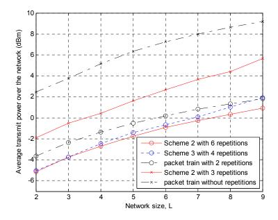
**Figure 15.** Average transmit power over the network depending on the number of nodes or the network size.
