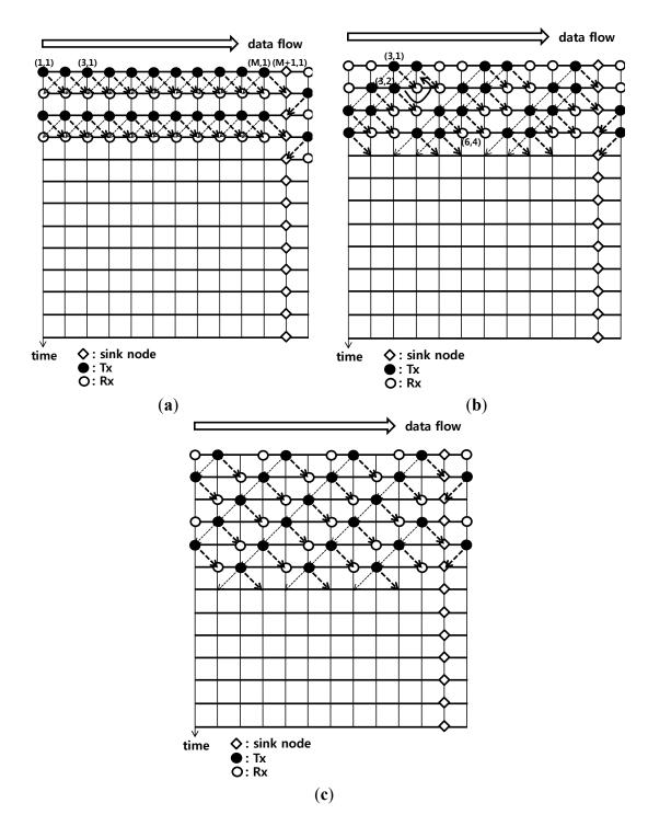
**Figure 4.** Proposed transmission/reception timing schemes. (The thick arrows represent data transfer) (**a**) Scheme 1; (**b**) Scheme 2; (**c**) Scheme 3.
