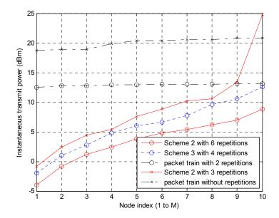
Figure 13. Transmit power of each node when the node is on the transmission state.
