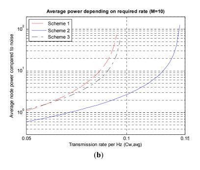
Figure 8. Average power depending on the transmission rates. (a) Wide range; (b) High rate range.
