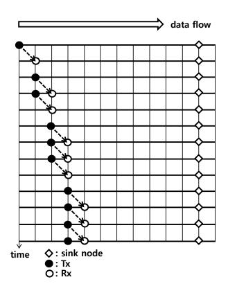
Figure 12. Transmission/reception timing of the packet train method.
