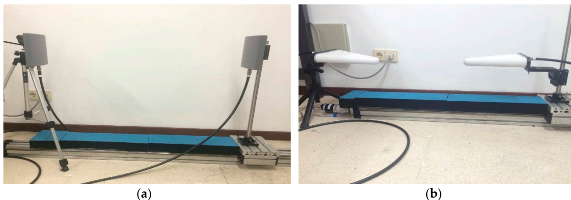
Figure 1. Path loss measurement system: (a) 868 MHz antenna setup; (b) 2.4/5.8 GHz antenna setup.
