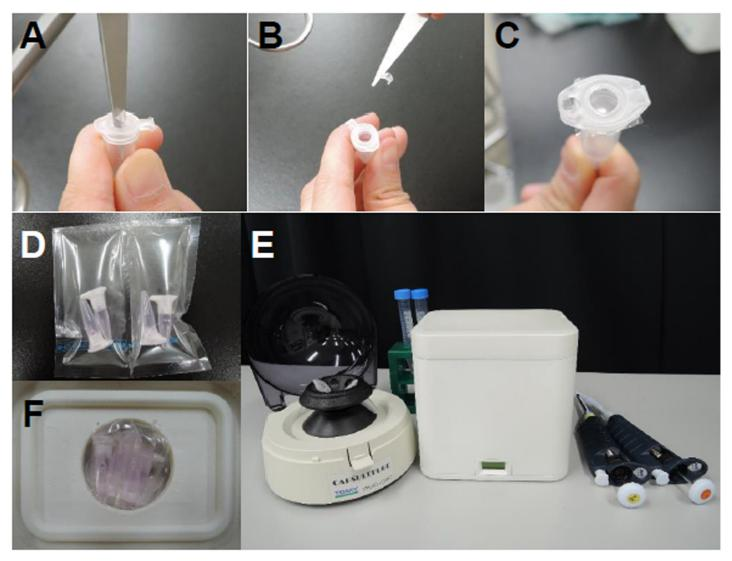
Fig 1. Microtubes and the simple warm box. (A) Puncturing a microtube lid using scissors. (B) A hole in the microtube lid facilitates gas exchange. (C) A microtube capped with a gas-permeable film. (D) Tubes were transferred into a plastic bag with the special gas mix. (E) Side view of the warm box showing a temperature indicator in the center. (F) A plastic bag placed in the box.
