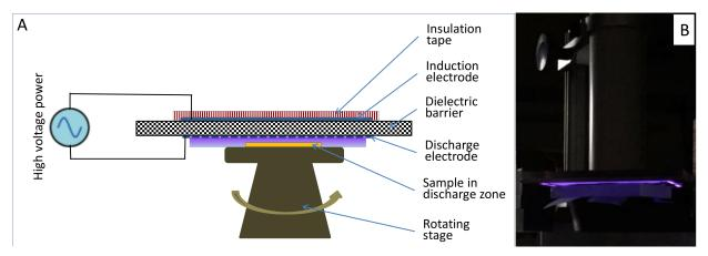
Figure 1. (A) Diagram of the NTP system and (B) photo showing a sample under glowing plasma discharge.
