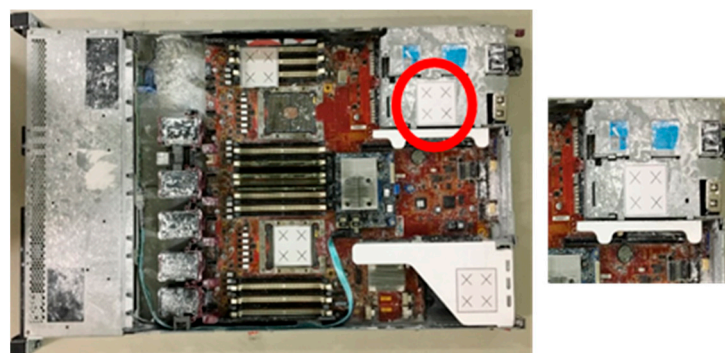
Figure 10. Object positioning system's target object with artificial markers. The red circle shows the artificial marker (square containing four crosses) used for positioning. The remaining three markers were used to analyze positional errors after camera shooting.
