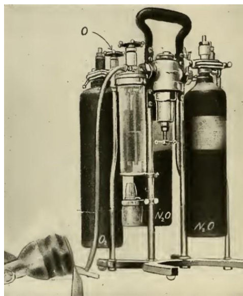
Figure 13 Gwathmey-Woolsey nitrous oxide-oxygen apparatus with cylinders attached. O, regulating valve for oxygen; O 2 , oxygen tank; N 2 O, nitrous-oxide tank. Observe bubble bottle. Original image from Gwathmey JT. Anesthesia. New York: Appleton; 1914.
