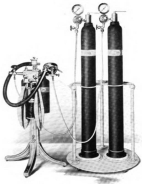
Figure 12 McKesson's apparatus, connected to cylinders of oxygen and nitrous oxide, which were used when the small gas tanks of the apparatus were exhausted. Public domain image. Courtesy of HathiTrust. Available at: https://babel.hathitrust.org/cgi/ptid=hvd.32044103003448&view=1up&seq=483 .
