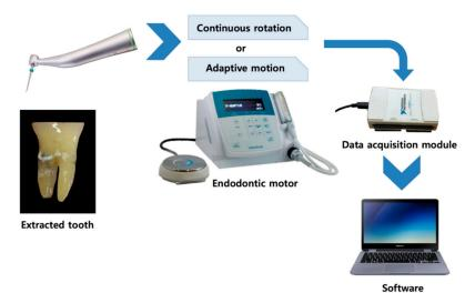
**Figure 1.** Diagram for test setup. Extracted teeth were used and two modes of kinetics of file movement were applied. The torsional load during instrumentation was recorded using a custom device and program.
