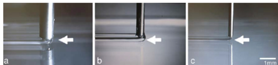
Figure 1. Images of printed hydrogels through (a) 20 ga, (b) 25 ga, and (c) 30 ga needle (Effect of nozzle diameter and dispensing speed on strands diameter), Reprinted with permission from Ref. [35], 2011, John Wiley and Sons.
