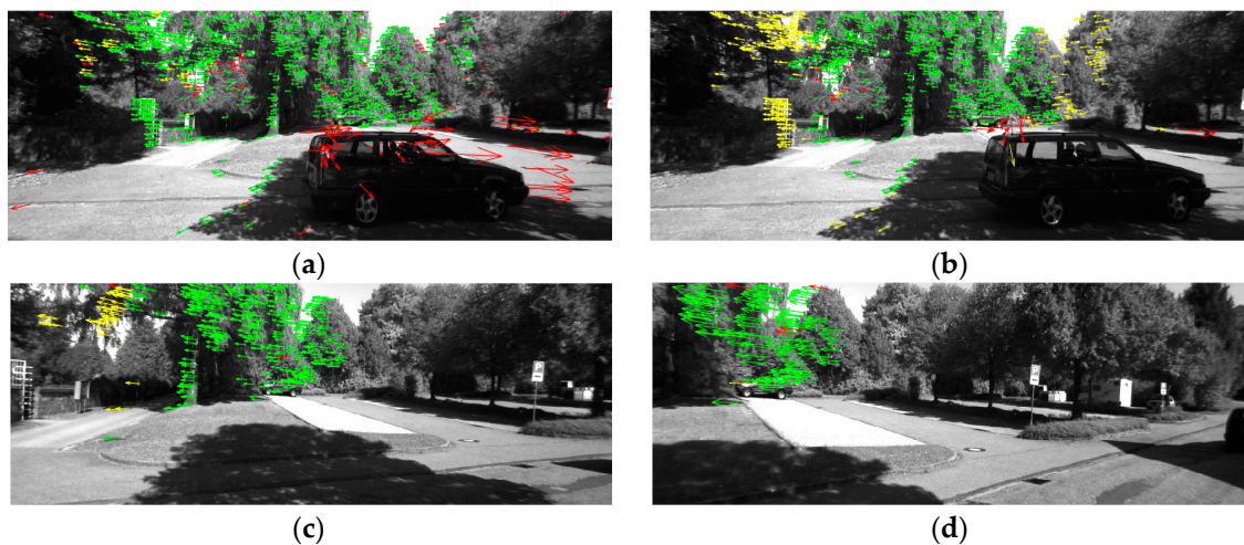
Figure 6. The feature points tracking results in scenario 2. (a) Frame 69; (b) Frame 70; (c) Frame 79; (d) Frame 89.
