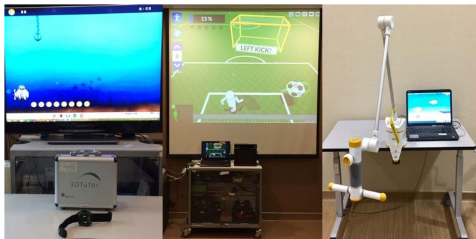
FIGURE 3. Technology-aided circuit training (left to right: Meditouch 3D Tutor wearable sensor for single-limb movement training, Jintronix Microsoft Kinect-based virtual reality platform to train full body movements, gait, balance and endurance capacities, Rejoyce to train upper limb functions focusing on prehension skills with proximal control [bilateral and unilateral training]).
