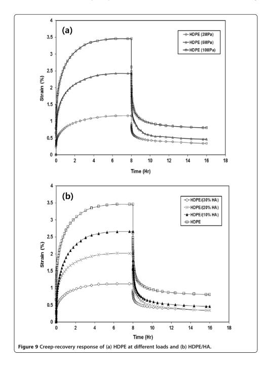
conditions. The improvement in the viscoelastic behavior due to gamma irradiation can be attributed to the crosslinking of HDPE chains that occurred in the amorphous region resulting in creation of rigid regions HDPE matrix [31].
