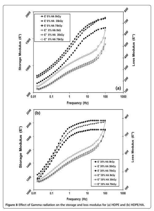
increase in the stiffness of polymeric matrix as a result of the decrease of free volume and the mobility restriction due to the presence of HA nanoparticles [17-19].
