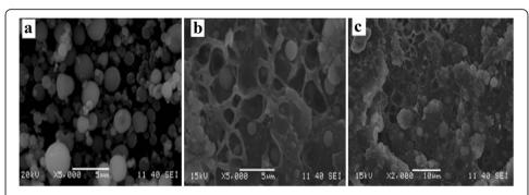
Figure 1 SEM micrograph of (a) HA nanoparticles (b) HDPE/HA nano composite 10% and (c) 30%.
