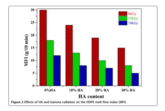
added to the polymer, the material viscosity increases and hence resistance to flow increases. Similar results have been also obtained where the MFI decreases due to irradiation and presence of HA for HDPE/HA (20:80) [29].
