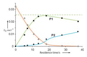
**Figure 4.** Effluent concentrations as a function of residence time of the hydrogenation of 3-methyl-1-pentyn-3-ol in ethanol over a 0.02 wt% Pd catalyst operated in segmented-flow at 24 °C. The dashed line shows the maximum obtainable yield.
