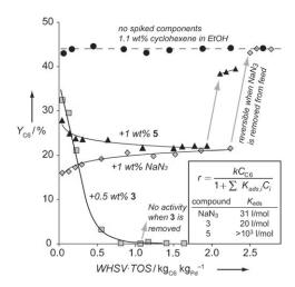
**Figure 5.** Spiking of cyclohexene hydrogenation at 24 °C with components from Scheme 2 to determine the strength and reversibility of adsorption on the Pd catalyst.
