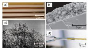
**Figure 2.** a) Darkening of a capillary after Pd impregnation (0, 1.1, 2.7, 5.7 wt % Pd); b) SEM micrograph of porous  $\gamma$ -Al<sub>2</sub>O<sub>3</sub> layer coated on the inner wall of the capillary; c) TEM micrograph of 5 nm Pd particles (black dots) supported on  $\gamma$ -Al<sub>2</sub>O<sub>3</sub> (5.7 wt % Pd); d) Formation of segmented flow at the capillary inlet.
