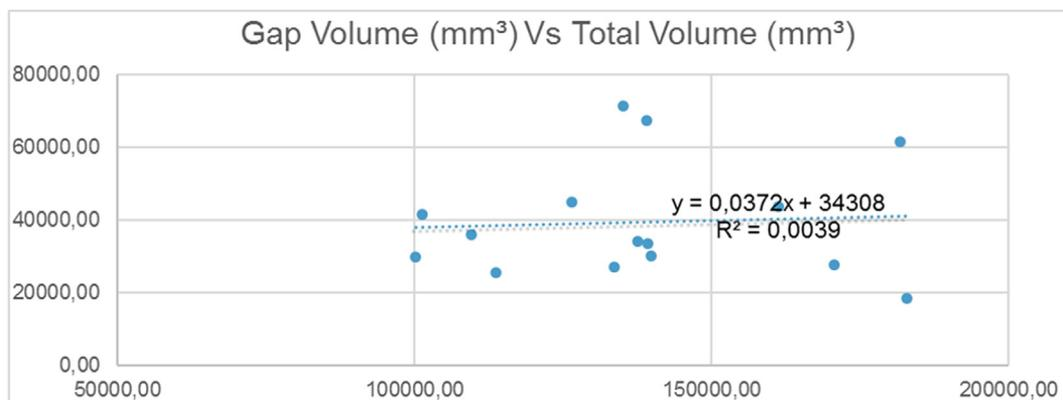
Fig. 8. Graph of the correlation between total volume and gap volume.
