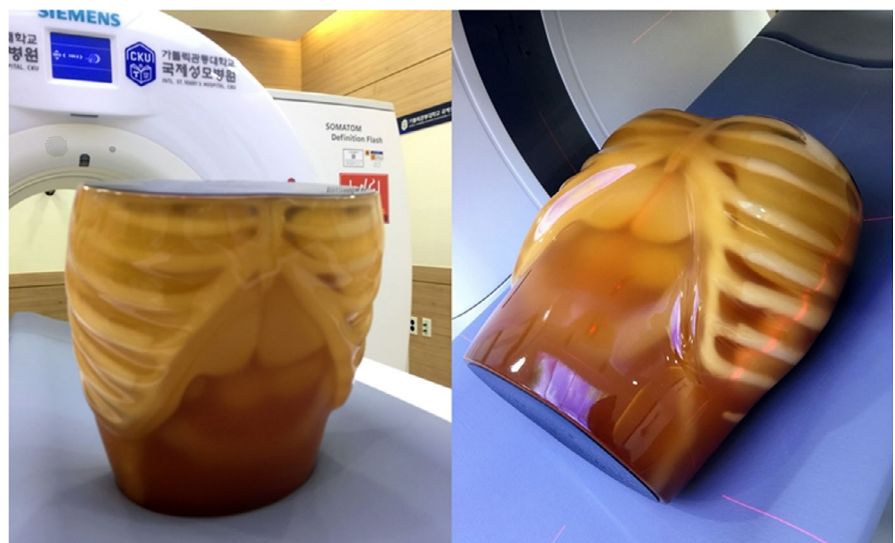
FIG. 1. Abdominal phantom for the experiment (phantom size: 25 \times 18 \times 28 \text{ cm}^3 ). (Kyoto Kagaku, Japan)
