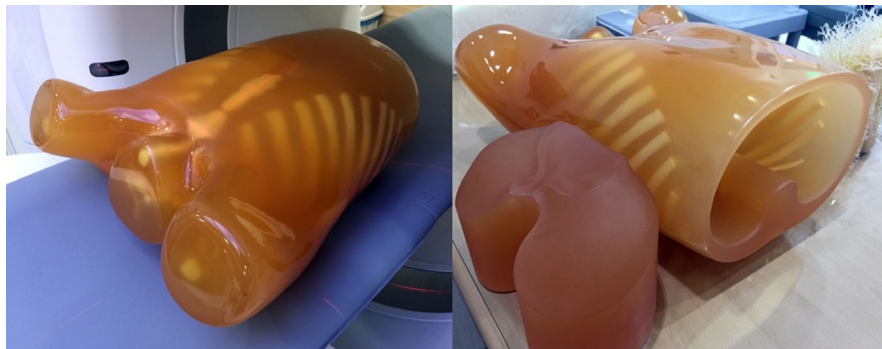
FIG. 3. Commercialized lungman phantom (phantom size: 43 \times 40 \times 48 \text{ cm}^3 , chest girth: 94 cm, weight: approx. 18 kg). (Kyoto Kagaku, Japan)
