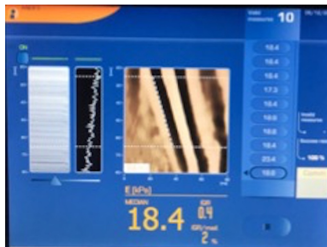
Fig 5. Fibroscan (Transient Elastography, TE). This figure illustrates the assessment of transient elastography on liver phantom 3. 10 valid elastography measurements are listed on the right side, where also success rate and invalid measurements are reported. The IQR/median is used as a quality parameter, and aimed to be below 30% while obtaining a success rate of at least 60%.
