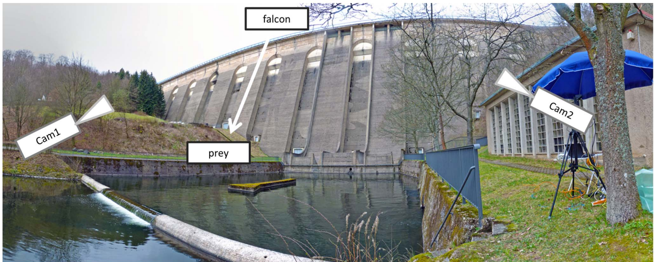
Figure 1. Experimental set-up in front of the dam wall (Olef-Talsperre, Hellenthal, Germany). The two cameras of the stereo system were positioned opposite, separated by a river leaving the dam wall. The features, displayed on the wall enabled us to calibrate the stereo camera system and to exactly determine the position of the diving falcon in the images of both cameras. doi:10.1371/journal.pone.0086506.g001
