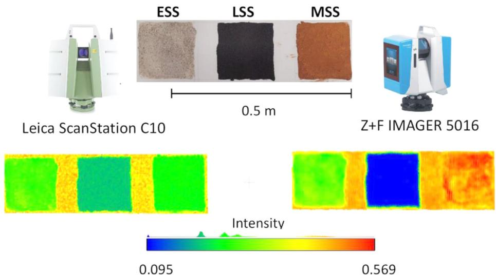
Fig. 1. Used scanners and specimens (modified from [6]).
