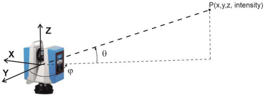
Fig. 2. Geometric data collected during the measurement by TLS.
