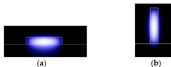
Figure 2. Fundamental mode in: (a) horizontal waveguide and (b) vertical waveguide.
