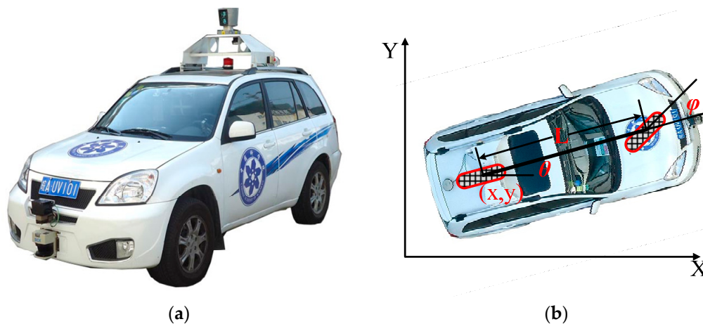
Figure 1. Autonomous vehicle prototype and its kinematic model. (a) "Intelligent Pioneer II" and (b) autonomous vehicle's bicycle model.
