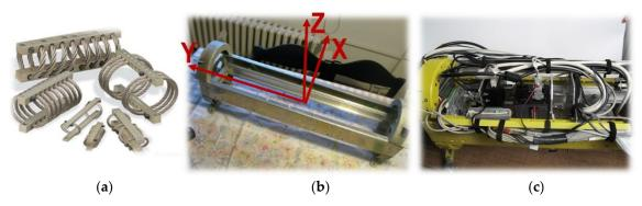
**Figure 9.** (a) Wire rope vibration dampers (ITT, 2019), (b) coordinate axes in sensor pod, (c) wire rope dampers installed in the sensor pod.
