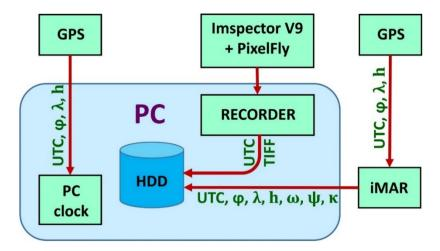
**Figure 7.** Schematic view of the integrated hyperspectral imaging system comprising ImSpector V9 + PixelFly camera.
