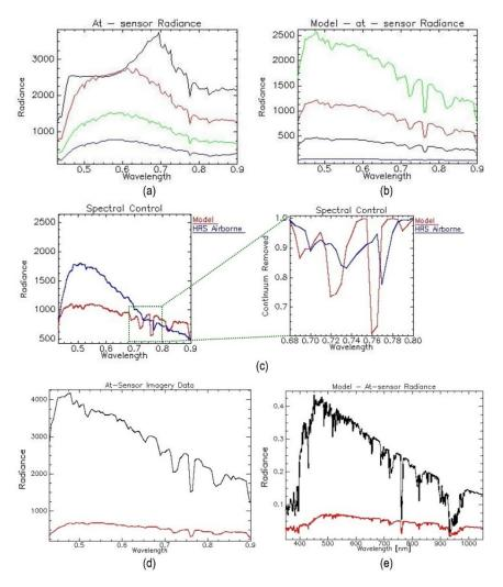
**Figure 12.** (a) Image at-sensor radiance and (b) modelled at-sensor radiance based on in situ measured reflectance (right side) of four selected ground targets. (c) Illustration of radiometric/spectral defects investigation of image spectral accuracy based on atmospheric gas absorption (blue spectrum) compared with simulated radiance (red) spectrum for the same ground-truth target. (d) The modelled at-sensor radiance based on in situ measured reflectance and (e) image at-sensor radiance.
