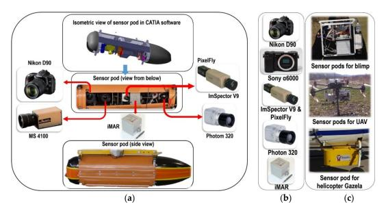
**Figure 8.** (a) Example of the first sensor pod designed and made with associated sensors for the Mi-8 and Bell-206 platforms. (b) Sensor used and (c) examples of a sensor pod designed and made for blimp (top), unmanned aerial vehicle (UAV, in the middle) and helicopter Gazela (bottom).
