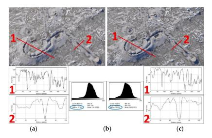
Figure 11. (a) Images ( $M_b \approx 1:12,000$ ) collected without damped vibrations with two profiles over the indicators of mine presence (trenches). (b) Passive damping of vibrations keeps the image sharper with two profiles over the indicators of mine presence (trenches). (c) Histograms of images with standard deviations (in blue ellipses).
