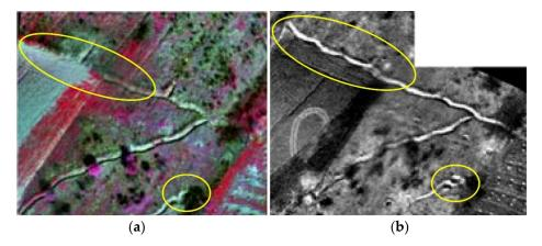
**Figure 14.** Examples of images of part of suspected hazardous area (from a height of 260 m,  $M_b \approx 1:10,800$ ) collected using sensors (a) multi-spectral VNIR and (b) panchromatic LWIR on which trenches can be seen (yellow ellipses).
