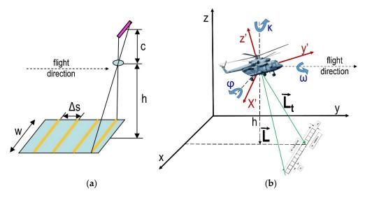
**Figure 5.** (a) Geometry of transference of the ImSpector V9 and PixelFly hyperspectral visible, near infrared (VNIR) systems, (b) transformation of theoretical view vector  $\vec{L}$  to effective view vector  $\vec{L}_t$ . κ, ω and φ denote roll, pitch and true heading angles respectively.
