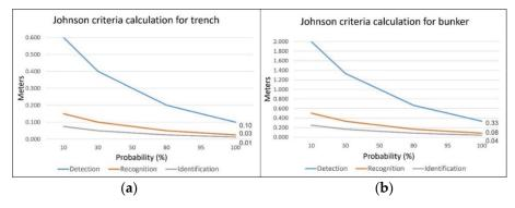
**Figure 15.** GDS size for the detection, recognition and identification of (**a**) a trench and (**b**) a bunker. Both diagrams show the GSD values for 100% detection, recognition and identification of the objects on the image.
