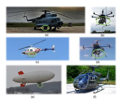
**Figure 3.** Platforms for aerial data acquisition system of AIDSS and sensor pods (in the green ellipses) on (a) Mi-8 helicopter, (b) remotely piloted aircraft system (RPAS) 8 ZERO, (c) Bell-206helicopter, (d) RPAS X8 MK, (e) blimp, and (f) Gazela helicopter.
