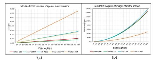
**Figure 13.** (a) Theoretical values of ground sample distance (GSD) of images of more significant AIDSS sensors for flight heights of 50 to 1000 m; (b) Theoretical values of image footprints of matrix sensors.
