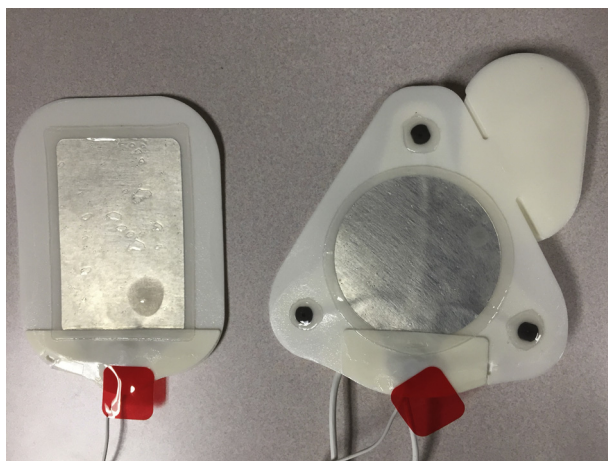
Figure 3 Comparison of the posterior (left) and anterior (right) patch electrodes. Note that the anterior patch electrode has multiple components, including a central, broad electrode for pacing, 3 button electrodes for sensing and pacing, and a heterogenous distribution of electrolyte-impregnated conductive semisolid.
