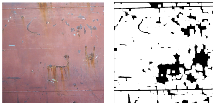
Figure 13. The result of UBE method after to process on a slice of 2 \times 2 m of ship's hull.
