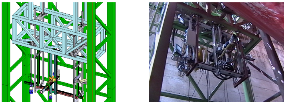
Figure 7. Attachment of the secondary structure.
