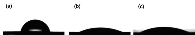
Fig. 4 Photographs of water morphology on the (a) PS, (b) CS and (c) prGO-CS membrane surfaces.
