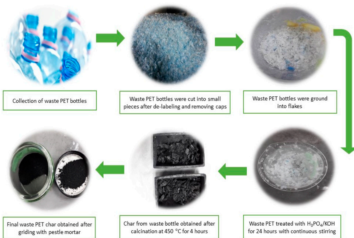
Figure 1. Synthesis of activated char from waste drinking bottles.
