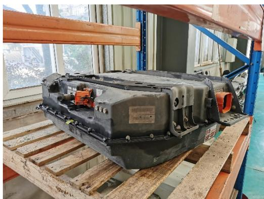
Figure 1.  $\text{LiFePO}_4$  electric vehicle (EV) battery pack.
