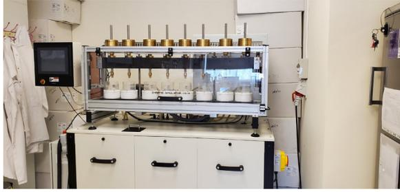
Fig. 1 – Chewing simulator CS-8, SD Mechatronik GmbH.
