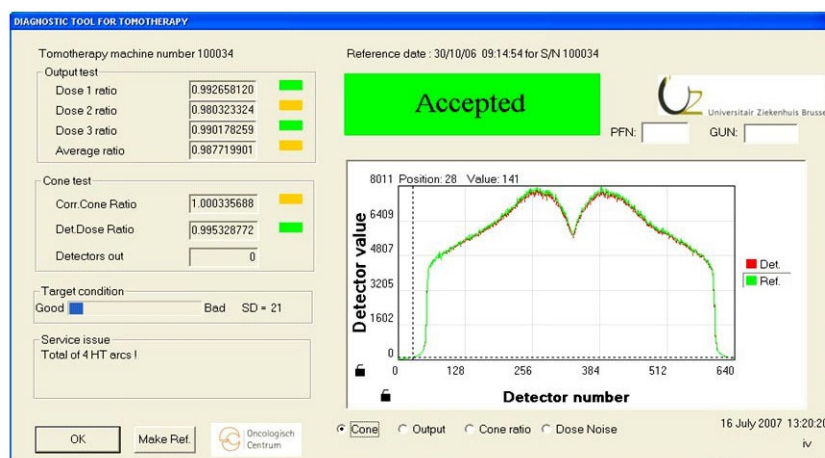
FIG. 1. The program layout of the tomocheck program. Five separate areas can be identified: output test, cone test, target condition, service issues, and the profile view area. The cone view is selected here. This profile is the average cone profile obtained by the detector during the whole treatment procedure together with the average cone profile of the reference.
