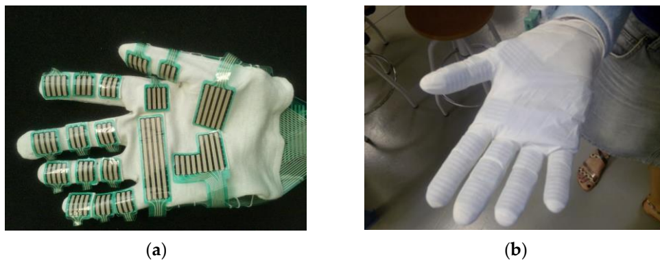
Figure 3. Pressure sensor sewn onto a cotton glove (a), final disposition in a subject's hand covered with the additional polyethylene and latex gloves (b).
