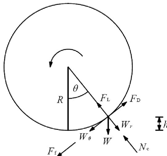
**Figure 24.** Stress analysis of the particle phase in the pipe wall area.
