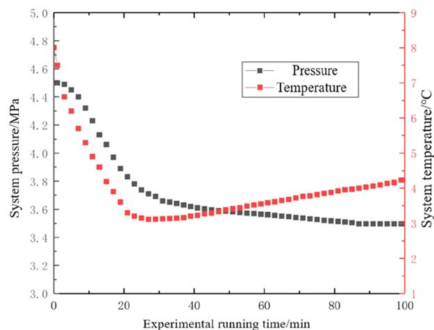
**Figure 15.** Temperature–pressure curve of hydrate formation and flow process in the pipeline (temperature, 3.5 °C; pressure, 4.5 MPa; moisture content, 15%; velocity of flow, 0.4 m/s; and twisted rate, 8.8).
