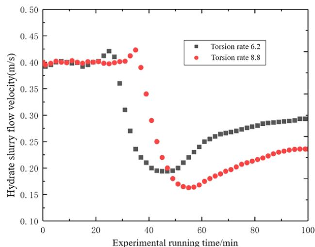
**Figure 16.** Velocity variation diagram of hydrate formation and flow process in the pipeline (temperature, 3.5 °C; pressure, 4.5 MPa; moisture content, 15%; and velocity of flow, 0.4 m/s).
