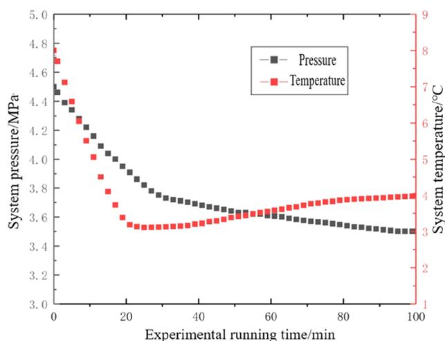
**Figure 7.** Temperature–pressure curve of hydrate formation and flow process in the pipeline (pressure, 4.5 MPa; moisture content, 15%; velocity of flow, 0.4 m/s; and twisted rate, 6.2).
