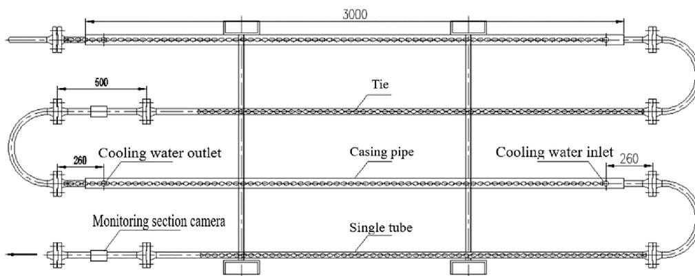
Figure 5. Structural diagram of the swirl flow hydrate generating unit.
