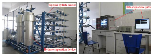
**Figure 1.** High-pressure hydrate formation flow experimental device.
