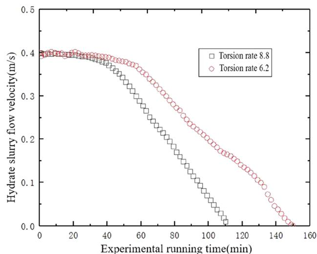
**Figure 20.** Variation in flow velocity during hydrate formation and flow in the pipeline (temperature, 4.5 °C; pressure, 3.5 MPa; moisture content, 25%; and velocity of flow, 0.4 m/s).
