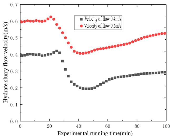
**Figure 12.** Variation of flow velocity during hydrate formation and flow in the pipeline (temperature, 3.5 °C; pressure, 4.5 MPa; moisture content, 15%; and twisted rate, 6.2).
