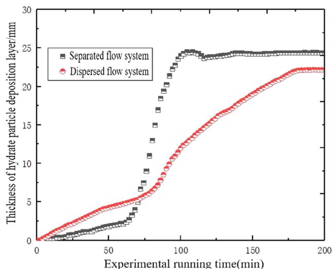
**Figure 21.** Variation law of hydrate particle deposition thickness (temperature, 4.5 °C; pressure, 3.5 MPa; moisture content, 25%; and twisted rate, 6.2).
