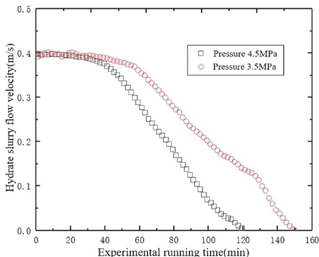
**Figure 19.** Variation in flow velocity during hydrate formation and flow in the pipeline (temperature, 4.5 °C; moisture content, 25%; velocity of flow, 0.4 m/s; and twisted rate, 6.2).
