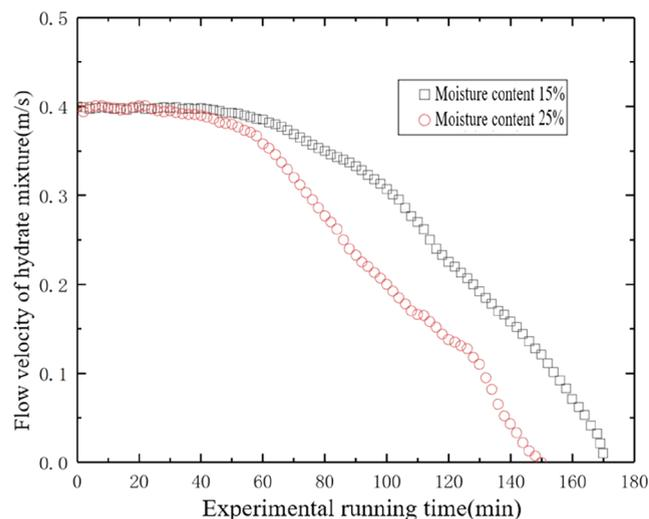
**Figure 17.** Variation in flow velocity during hydrate formation and flow in the pipeline (temperature, 4.5 °C; pressure, 3.5 MPa; velocity of flow, 0.4 m/s; and twisted rate, 6.2).
