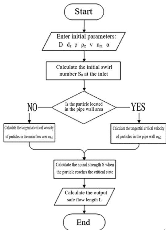
Figure 25. Calculation flow chart of hydrate particle safety distance in the swirl flow system.
