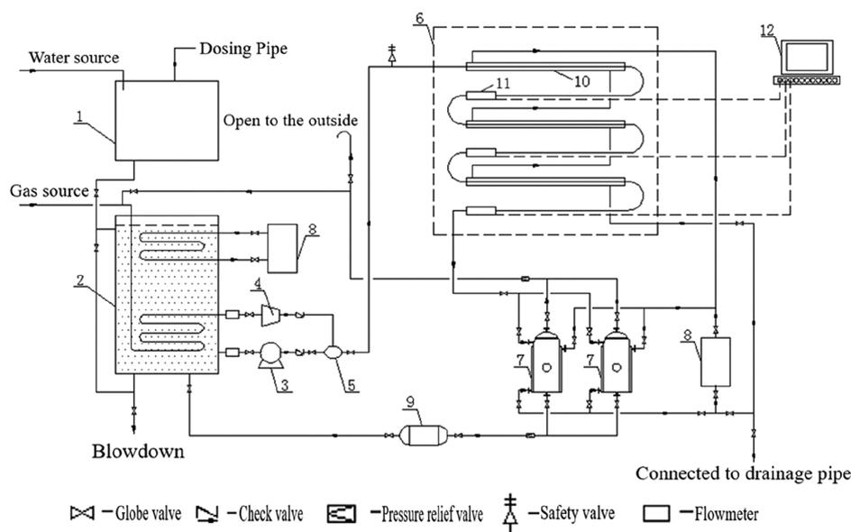
Figure 4. Flow chart of the high-pressure hydrate experiment loop. (1) Water tank, (2) low-temperature water tank, (3) magnetic pump, (4) booster pump, (5) mixer, (6) generating unit, (7) separator, (8) cold water bath, (9) buffer tank, (10) bushing, (11) monitoring pipe section, and (12) data acquisition device.
