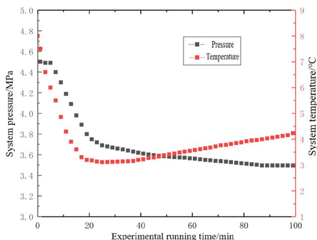
**Figure 9.** Temperature–pressure curve of hydrate formation and flow process in the pipeline (pPressure, 4.5 MPa; moisture content, 25%; velocity of flow, 0.4 m/s; and twisted rate, 6.2).
