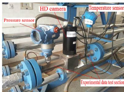
Figure 2. Experimental data test section.
