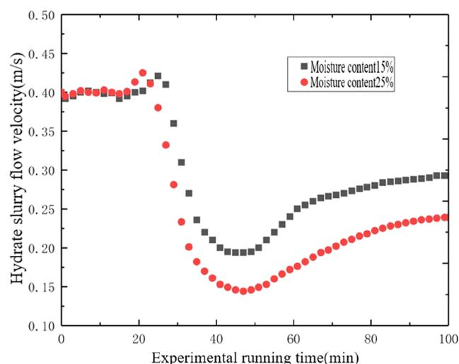
**Figure 10.** Variation of flow velocity during hydrate formation and flow in the pipeline (pressure, 4.5 MPa; velocity of flow, 0.4 m/s; and twisted rate, 6.2).
