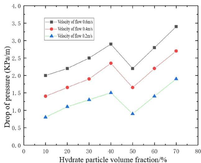
**Figure 22.** Variation in pressure drop with hydrate volume fraction at different flow rates (temperature, 4.5 °C; pressure, 3.5 MPa; moisture content, 25%; and twisted rate, 6.2).
