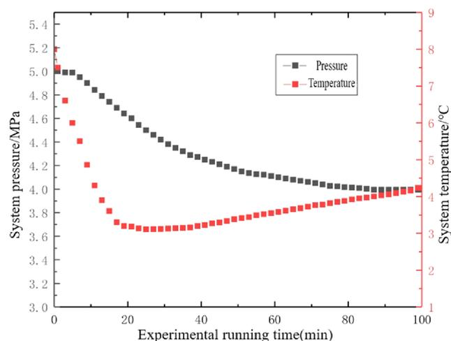
**Figure 13.** Temperature–pressure curve of hydrate formation and flow process in the pipeline (temperature, 3.5 °C; pressure, 5 MPa; moisture content, 15%; velocity of flow, 0.4 m/s; and twisted rate, 6.2).
