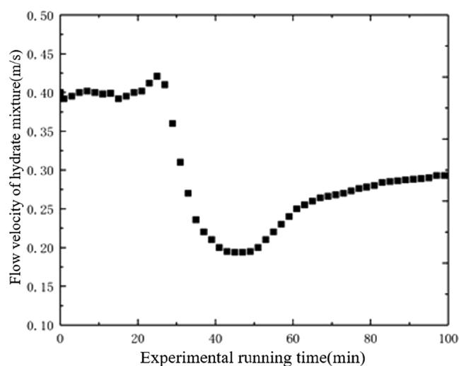
**Figure 8.** Variation of flow velocity during hydrate formation and flow in the pipeline (pressure, 4.5 MPa; moisture content, 15%; velocity of flow, 0.4 m/s; and twisted rate, 6.2).
