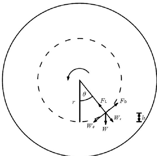
**Figure 23.** Stress analysis diagram of particle phase in the main flow area.
