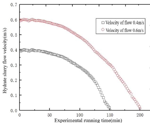
**Figure 18.** Variation in flow velocity during hydrate formation and flow in the pipeline (temperature, 4.5 °C; pressure, 3.5 MPa; moisture content, 25%; and twisted rate, 6.2).
