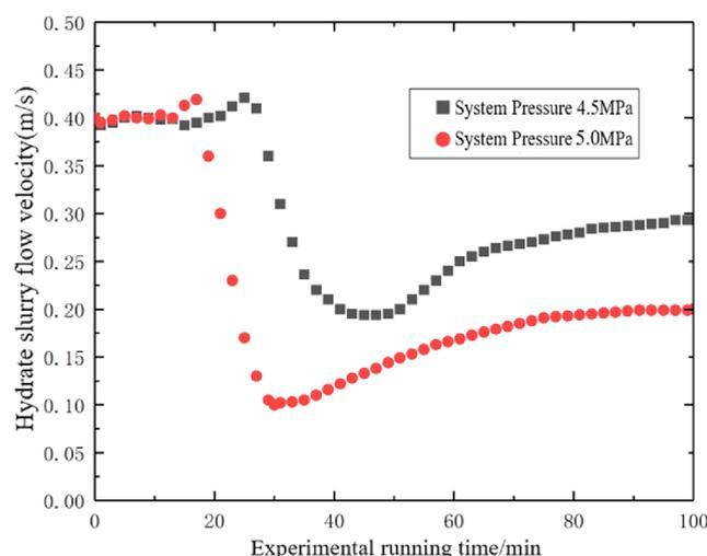
**Figure 14.** Variation in flow velocity during hydrate formation and flow in the pipeline (temperature, 3.5 °C; moisture content, 15%; velocity of flow, 0.4 m/s; and twisted rate, 6.2).
