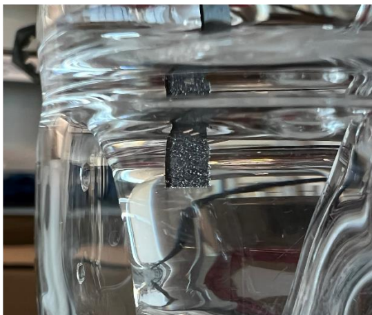
Figure S 41. \text{NO}_3\text{RR} electrolysis over (a) Ru-N-C and (b) Rh-N-C, showing gaseous bubbles produced on the working electrode. Demonstrating the Ru/Rh-N-C catalysts being out competed by the HER, yielding a large gap in the GAP of Figure 4 and Figure S 38.
