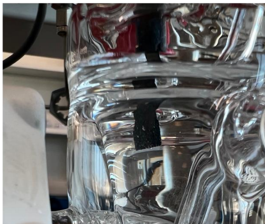
Figure S 41. \text{NO}_3\text{RR} electrolysis over (a) Ru-N-C and (b) Rh-N-C, showing gaseous bubbles produced on the working electrode. Demonstrating the Ru/Rh-N-C catalysts being out competed by the HER, yielding a large gap in the GAP of Figure 4 and Figure S 38.
