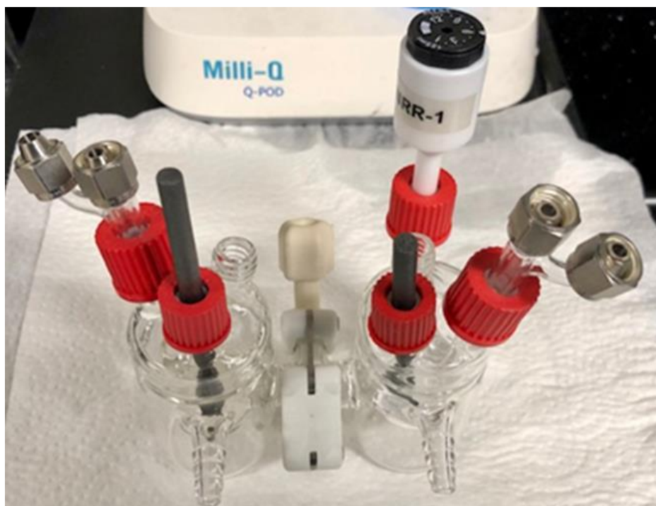
Figure S 66. Electrochemical H-cell used in this work. Left hand side is the counter chamber with the graphite counter working electrode. The right-hand side contains the RHE reference electrode (in a separate chamber connected through a glass frit) and graphite rod with the carbon paper working electrode. The septum on both the left and right hand side allow for gas inlet and outlet into the working and counter chambers.
