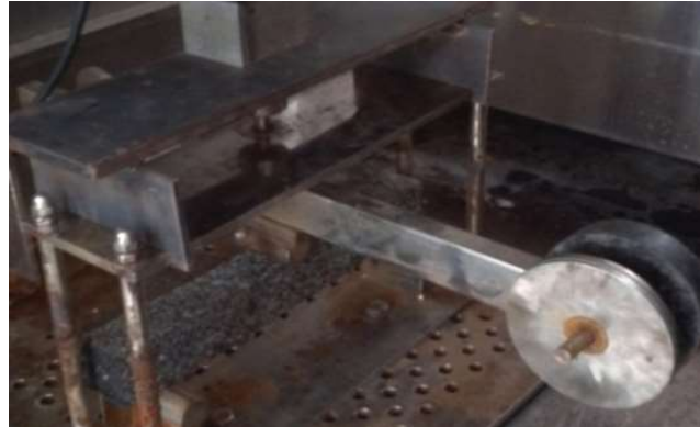
Figure 5. Bending creep test.
