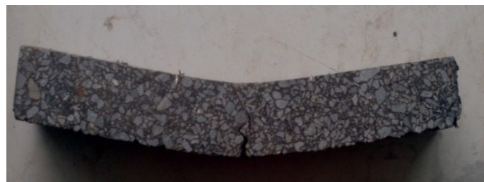
Figure 3. Specimen for bending creep test.
