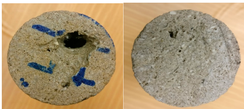
Figure 11. Images for the core inlet (left) and outlet (right) for the high- permeability sample after thermochemical/HCl treatment.
