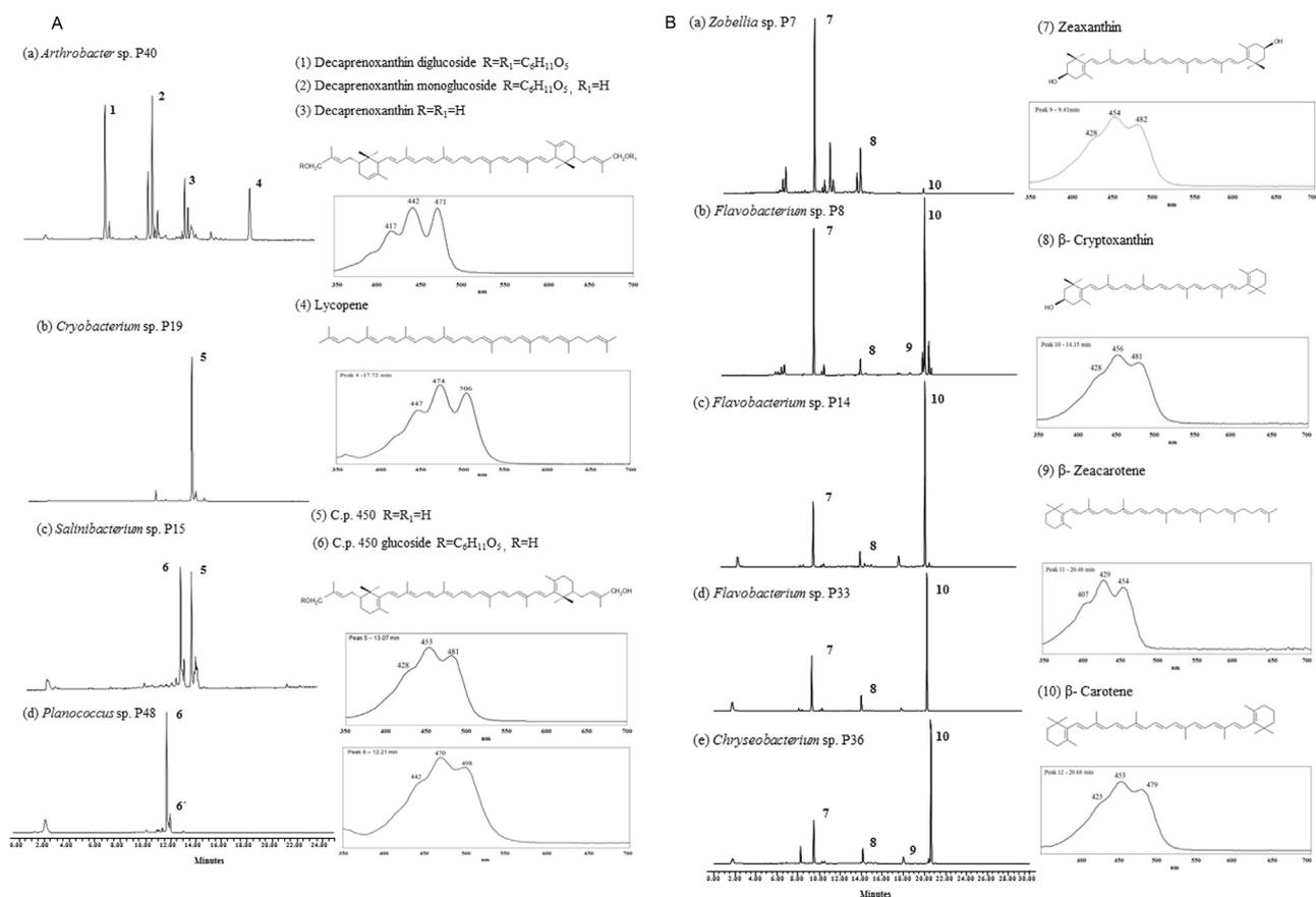
**Fig. 1.** Reversed-phase HPLC-DAD chromatograms at 450 nm and UV-vis spectra of the carotenoid extracts of the bacteria strains. (A) C50 carotenoids, (B) C40 carotenoids.
