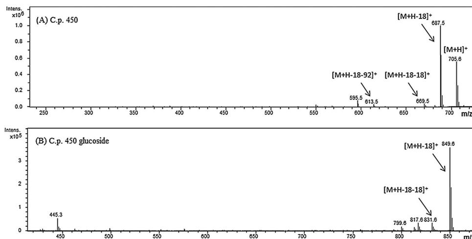
Fig. 2. Mass spectra of (A) C.p. 450 and (B) C.p. 450 glucoside in atmospheric pressure chemical ionization (APCI) in positive mode.
