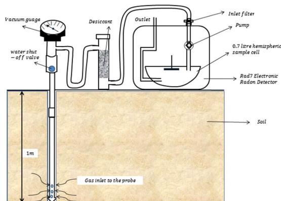
**Figure 2.** Experimental set-up for radon-in-soil gas measurement (Source: Ajiboye *et al.* 2018). The set-up involves three main components which are (i) the RAD7 electronic radon detector which detects and measures radon concentration, (ii) the desiccant which is a column of  $\text{CaSO}_4$  which eliminates moisture from gas going into the RAD7, and (iii) soil gas probe which is inserted into the soil for radon gas collection.
