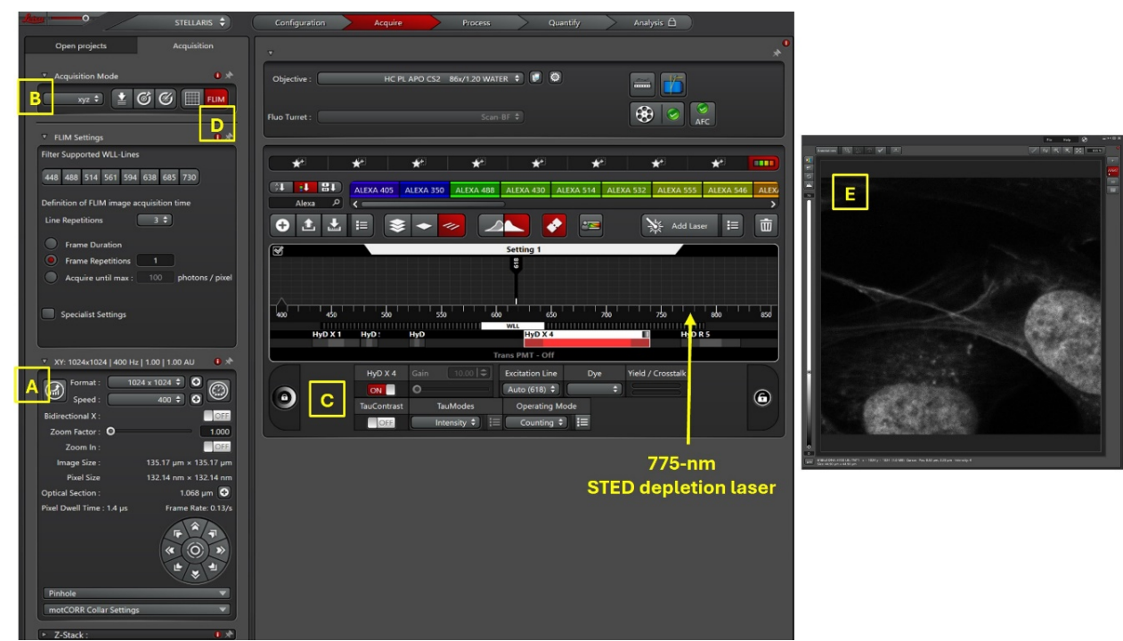
Figure 1. Screenshot of LAS X software for image acquisition of three dyes simultaneously. In this example, three probes (SPY620-DNA, SiR700-Act, and LBL-Dye M715), indicated by * in Table 1, are acquired in one single detector after 618 nm laser excitation (5% WLL laser power). The confocal image, on the right side, shows one color image for the three dyes.
