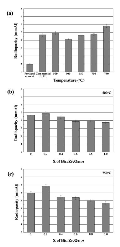
**Figure 11.** (a) Comparison of radiopacity of heat-treated  $Bi_{1.8}Zr_{0.2}O_{3.1}$  powders and commercial ceramic materials. Radiopacity of various  $Bi_{2-x}Zr_xO_{3+x/2}$  powders after heat treatment at: (b) 500 °C; and (c) 750 °C.
