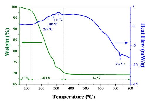
Figure 1. DSC/TGA analytic results of the as-synthesized sol-gel Bi<sub>2</sub>O<sub>3</sub> powders.
