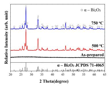
Figure 2. XRD patterns of as-obtained and heat-treated Bi<sub>2</sub>O<sub>3</sub> powders prepared using the sol-gel process.
