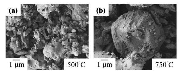
**Figure 3.** SEM images of sol-gel Bi<sub>2</sub>O<sub>3</sub> powders after heat-treatment at: (a) 500 °C; and (b) 750 °C.
