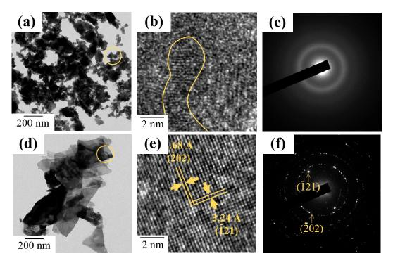
**Figure 4.** TEM images of sol-gel  $Bi_2O_3$  powders (a) before and (d) after 500 °C heat treatment. (b,e) HRTEM images; and (c,f) selected area diffraction pattern (SAED) taken from the circled area in (a,d), respectively.
