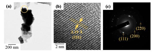
**Figure 10.** (a,b) TEM images and (c) SAED pattern of  $Bi_{1.0}Zr_{1.0}O_{3.5}$  powders after heat treatment at 750 °C.
