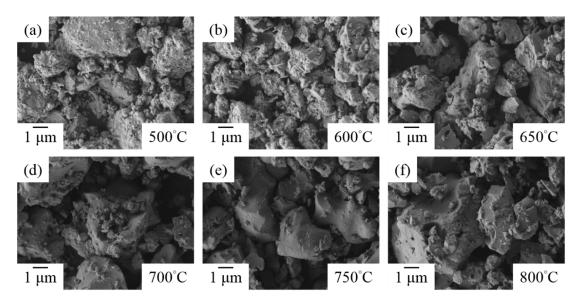
**Figure 7.** SEM images of  $Bi_{1.8}Zr_{0.2}O_{3.1}$  powders after heat treatment at temperatures of: (a) 500 °C; (b) 600 °C; (c) 650 °C; (d) 700 °C; (e) 750 °C; and (f) 800 °C.
