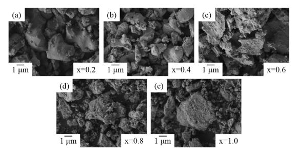
**Figure 8.** SEM images of  $Bi_{2-x}Zr_xO_{3+x/2}$  powders after 750 °C heat treatment at: (a) x = 0.2; (b) x = 0.4; (c) x = 0.6; (d) x = 0.8; and (e) x = 1.0.
