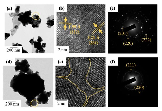
**Figure 9.** TEM images and SAED patterns of (**a–c**)  $Bi_{1.8}Zr_{0.2}O_{3.1}$  and (**d–f**)  $Bi_{1.0}Zr_{1.0}O_{3.5}$  powders after heat treatment at 500 °C.
