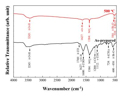
**Figure 5.** FT-IR spectrum of as-obtained and heat-treated Bi<sub>2</sub>O<sub>3</sub> powders prepared using the sol-gel process.
