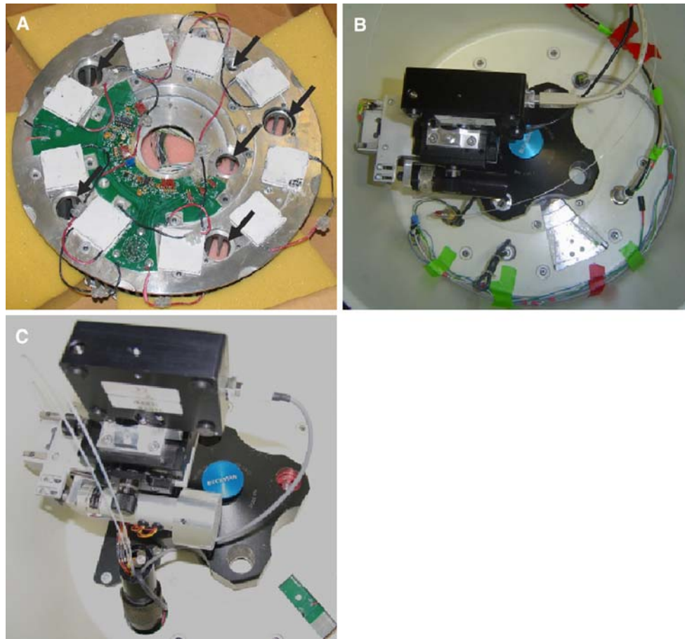
Fig. 1 a XI-heatsink with six additional holes (indicated by arrows ) drilled in as optical channels or for mounting optical or electric vacuum feeds. b The same heatsink mounted in a XL preparative ultracentrifuge with multiwavelength detector. c Multiwavelength detector mounted on an XL-I heatsink
