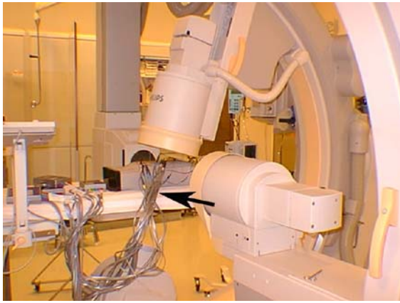
Fig. 4 Five-year-old anthropomorphic phantom and MOSFET dosimeters with leads ( arrow ) in the cardiac angiography laboratory
