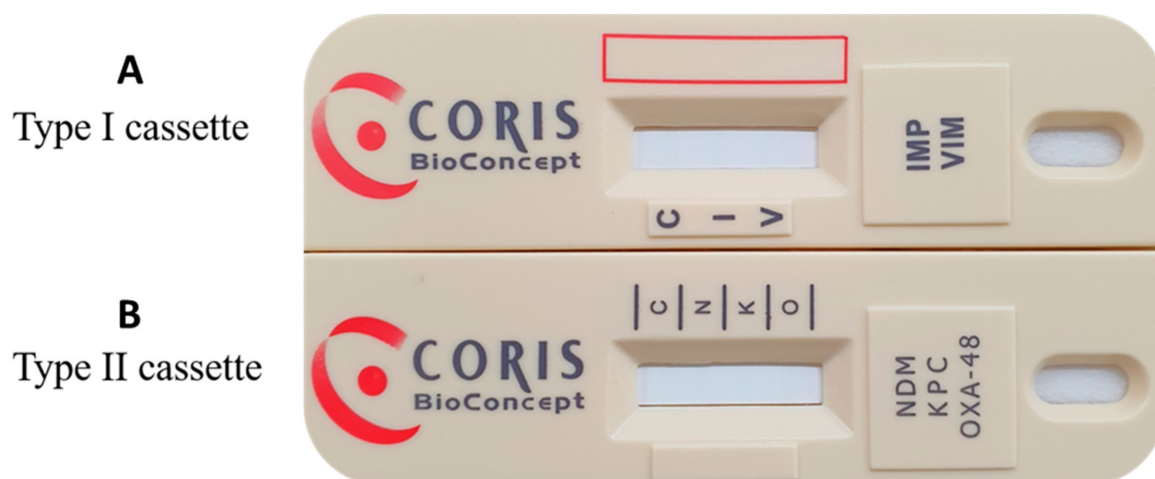
Figure 1. Two lateral-flow cassettes. Each cassette contains one sensitized strip. (A) The type I cassette contains a nitrocellulose membrane sensitized with monoclonal antibody directed against IMP carbapenemase (“I” line) and VIM carbapenemase (“V” line) and a control capture reagent (“C” line). (B) The type II cassette contains a nitrocellulose membrane sensitized with monoclonal antibody directed against NDM carbapenemase (“N” line), KPC carbapenemase (“K” line) and OXA-48-like carbapenemase (“O” line) and a control capture reagent (“C” line).
