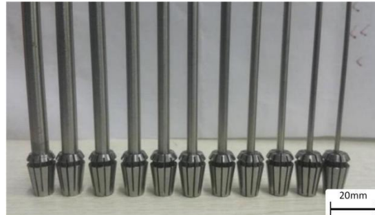
Figure 7. The different diameters of the rotating rods in the experiment.
