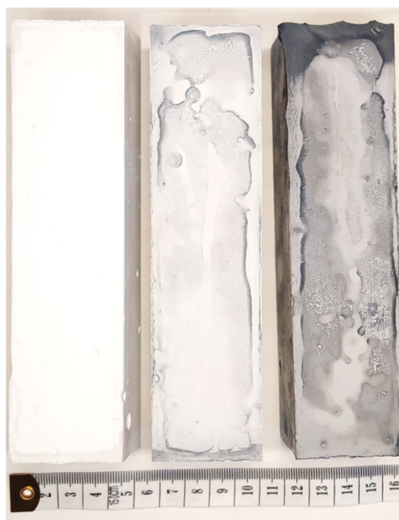
Figure 3. 28-days specimens: MOC-REF, MOC-GO-OMWCNT-0.1, MOC-GO-OMWCNT-0.2 (from left).
