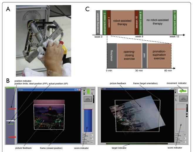
**Figure 1 The HapticKnob robot and the proposed therapy protocol**. A: Stroke subject training on the HapticKnob. B: Visual feedback of the opening/closing (left) and pronation/supination (right) exercises, where subjects have to squeeze, respectively orient the picture into a white frame by grasping, respectively turning the *HapticKnob*. C: Details of therapy and session protocol.
