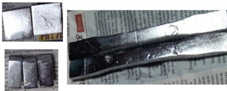
Figure 5. Electroless nickel-plated PETG+MWCNT specimens.
